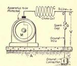
Fig. 151.—The principle of the lightning protector.
